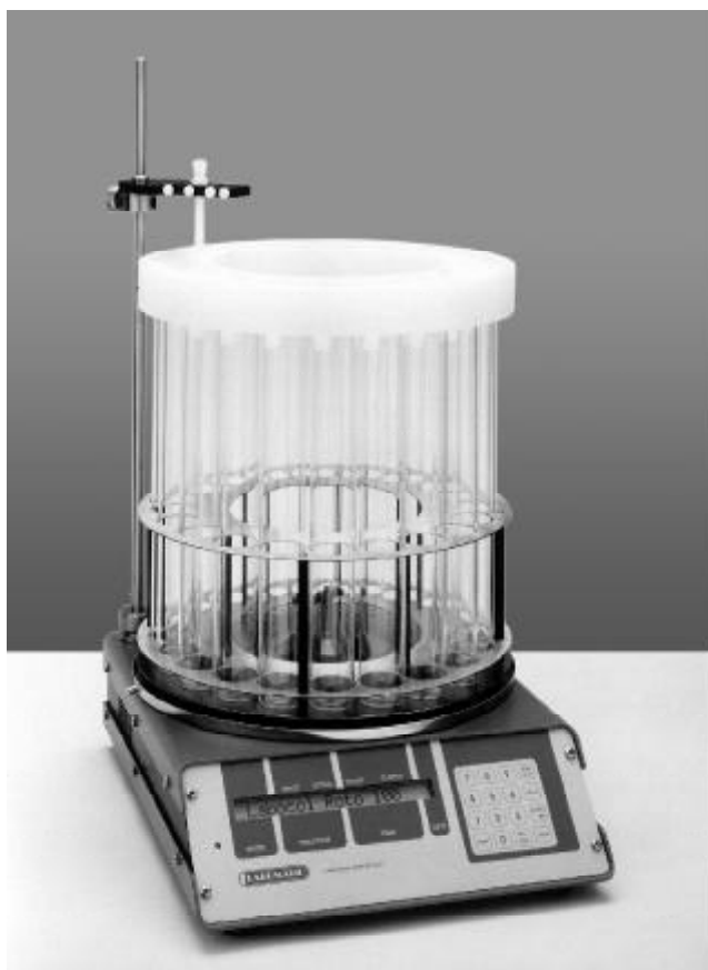
LABOCOL Roto-100 with preparative/large volume rack and large volume vials
